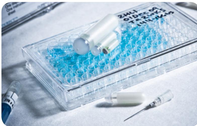
Besides offering the benefit of continuous and direct delivery of nanoparticles, ALZET pumps are themselves an embodiment of nanotechnology. With more than 35 years of research behind the technology, the pump's nanoporous, semipermeable membrane represents one of the most reliable approaches for continuous delivery of biological agents to small lab animals. Its small size, simple design, controlled delivery, and ease of use,
