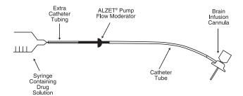
Step 7. Fill the osmotic pump with the solution to be delivered, using the recommended procedure described in the ALZET Osmotic Pump Instruction Sheet. Ascertain that the fill volume is greater than or equal to the volume specified on the instruction sheet for that model.
